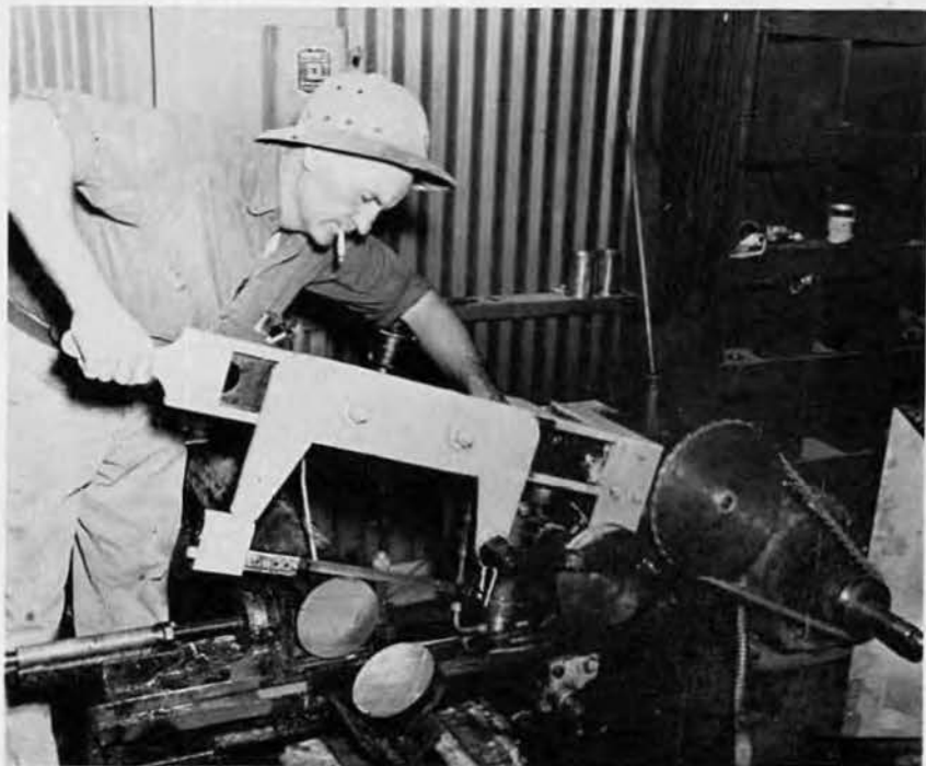
Above: Ingenious Swoboda also improvised a power hack-saw for some hard cutting.
